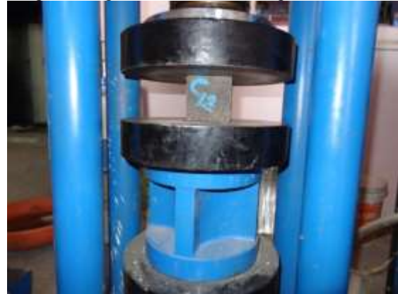
Fig 4 Setup of Compressive strength test
