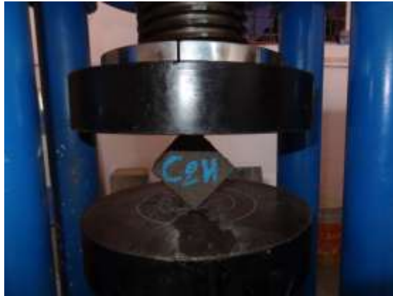
Fig 5 Setup of Splitting tensile strength
